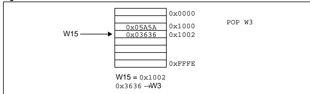
Figure 2-7: Stack Pointer After a POP Instruction
