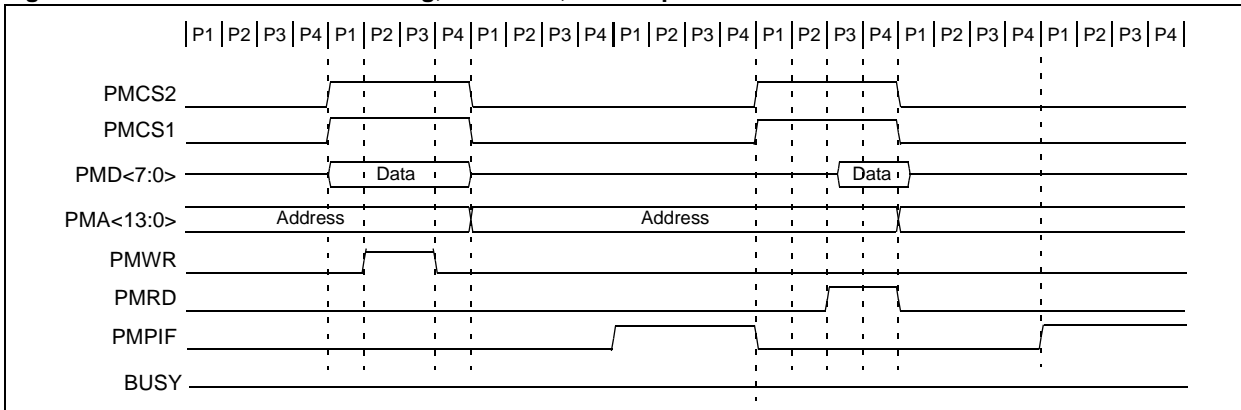
Figure 13-13: Read and Write Timing, 8-Bit Data, Demultiplexed Address
